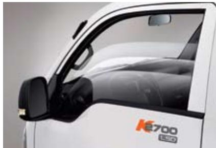
**Power windows & Outside mirror with side repeater:** Operate smoothly at the touch of a button mounted on the door armrest and OSR(Outside mirror with side repeater) is an option limited to the LHD countries within the general region.
